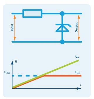
Using a Zener diode for output voltage stabilization
