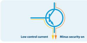
The transistor controls large current by means of low one
