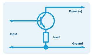
Connection diagram for a bipolar common-collector transistor
