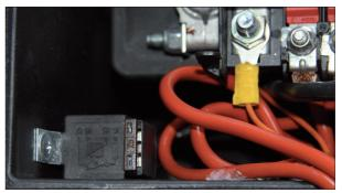
Connecting a load to the storage battery via a relay and fuses
