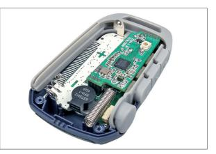
Example of antenna built into the remote control unit
