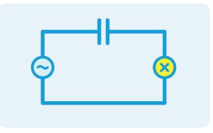
**Capacitor and alternating current**
