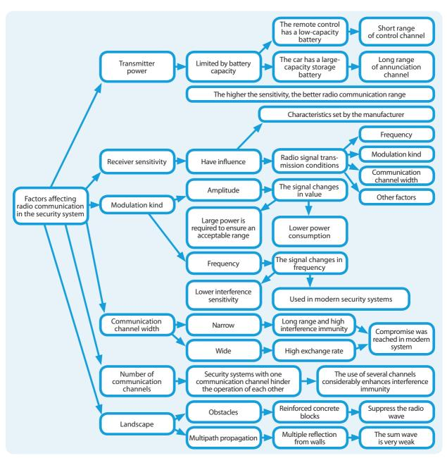
Radio control of the security system. Memo diagram
