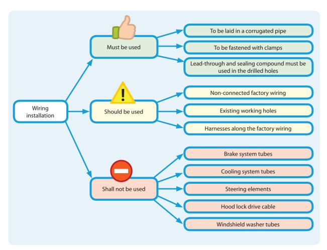
Wiring installation. Memo diagram
