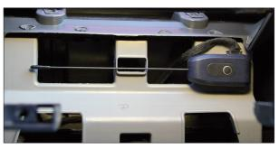
Transceiver module under the dashboard cover plate
