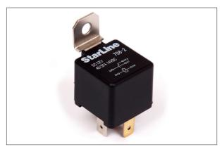
The relay consists of two main parts — a winding with core (electromagnet) and a group of contacts. Both these parts are joined in one package. When voltage occurs on the winding, one of the relay contacts is attracted to the electromagnet and is closed with the other one. Simultaneously, opening with the third contact may occur.
