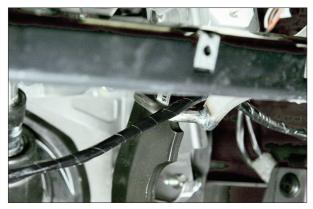
Poor quality of security system installation: wires are not fastened
