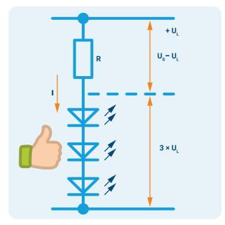
**Correct connection diagram of LEDs**
