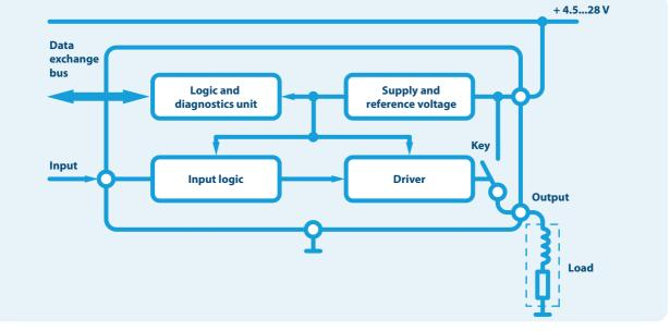
Standard structural diagram of the smart switch
