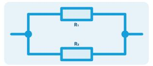
Parallel connection of resistors
