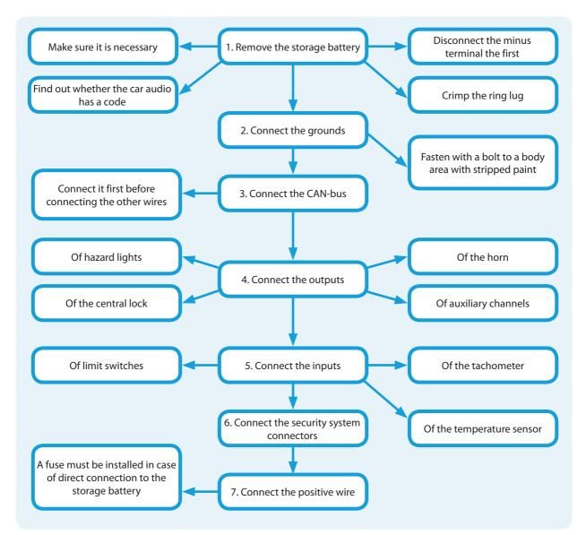
Procedure for connection of security system elements. Memo diagram
