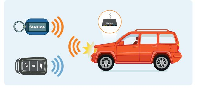
intruder has no tag, the car will be immobile and the horn will be sounding. In case of this authorization method, radius of tag recognition is 5-20 meters and can be adjusted during installation.
