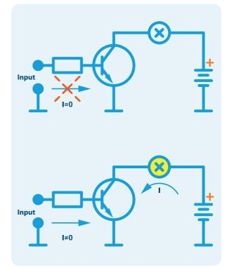
Transistor operation as a switch
