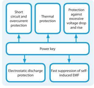
Power switch structural diagram
