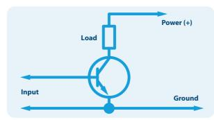
Connection diagram for a bipolar common-emitter transistor
