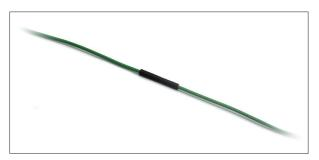
**4.** Move the heat-shrink tube to the soldering area.
