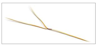
**4.** Pass a single wire between the strands and wrap the first wire with it
