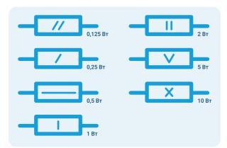
Designation of resistor dissipation power in the diagram
