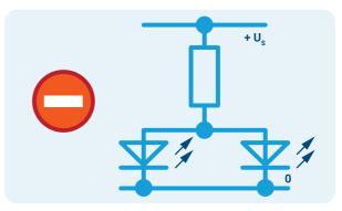
Incorrect parallel connection diagram of LEDs
