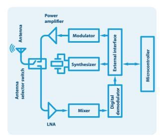
Structural diagram of digital transceiver
