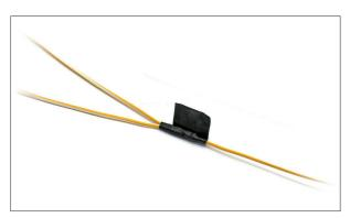
Improper insulation of the connection - free ends of the insulating tape are left
