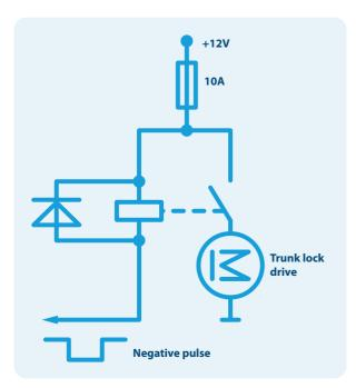
Using an additional relay for trunk unlocking
