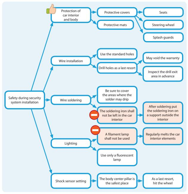
Safety during security system installation. Memo diagram
