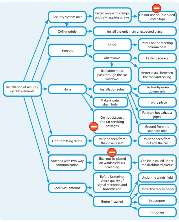
Installation of security system elements. Memo diagram
