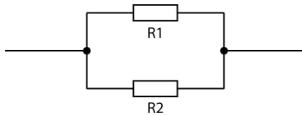
$$R_{\text{общ}} = (R_1 \cdot R_2) / (R_1 + R_2)$$
